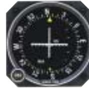
Has pivoted needle action and plastic lens. Internal blue-white lighting.
