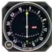
**KI 208 VOR/LOC Indicator.** Has a self-contained VOR/LOC converter for use with the KX 155. Left/right course deviation is displayed.
