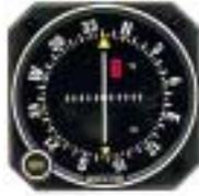
**KI 202/KI 203 VOR/LOC Indicators.** The KI 202 is compatible with the KX 165 without glideslope or other NAV systems which contain their own VOR/LOC converters. The KI 203 is compatible with the KX 155 or other NAV systems which do not contain their own VOR/LOC converter. Both indicators feature rectilinear needle action for left/right course deviation, anti-reflective coated lens, and internal blue-white lighting.
