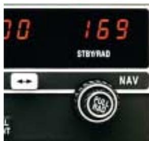
The lower-cost KX 155 system is virtually identical in appearance to the KX 165; however, it doesn't include the digital Radial readout feature. Also, the KX 155 requires an external VOR/LOC converter (usually included in the appropriate Bendix/King NAV indicator) while the KX 165 comes with a built-in VOR/LOC converter designed to interface directly with any ARINC standard CDI or HSI display.
