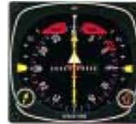
**KI 525A Horizontal Situation Indicator.** As the panel display for the KCS 55A Slaved Gyrocompass System, this indicator combines heading and VOR/LOC deviation information in a single pictorial presentation of the complete navigation situation. It is compatible with the KX 165 (with GS) or other NAV systems with built-in VOR/LOC converters. This instrument also provides glideslope deviation display plus course and heading outputs for Autopilots and Flight Directors.
